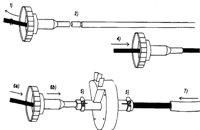
1/ Choose a straight location for the sensor where it will not be damaged by heat or vibration. Note the length of inner cable which protrudes from the outer sheath so that this can be replicated when the sensor and cable assembly is completed.
